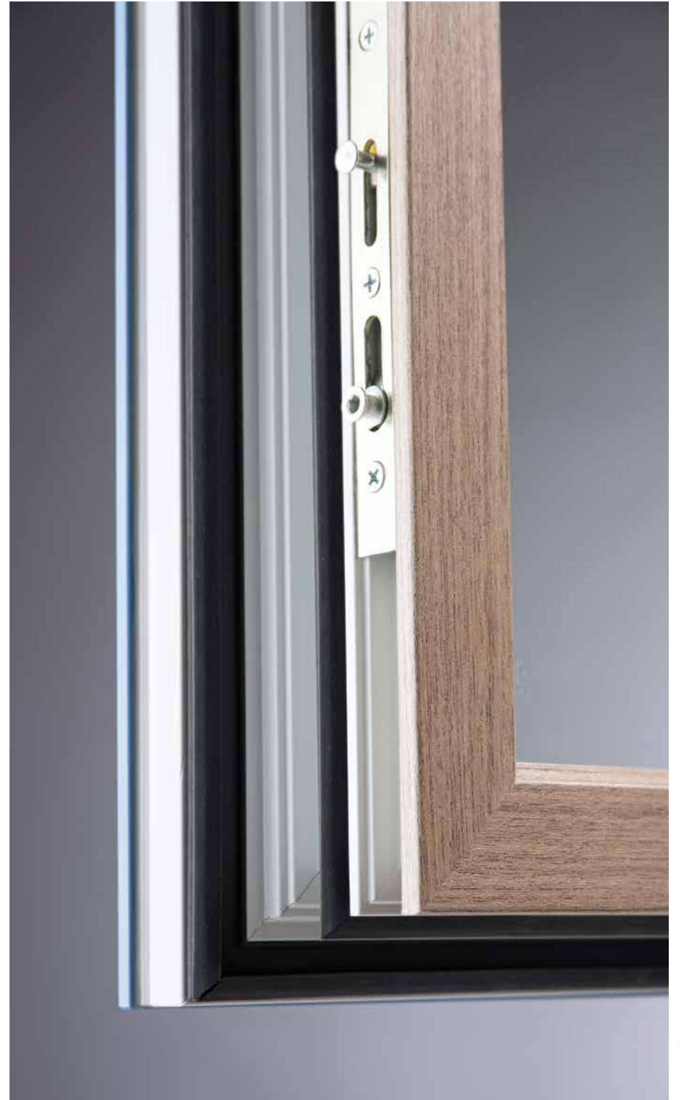
80mm double rebate with triple seal and Winkhaus locking system
